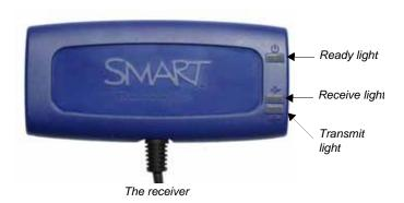
To avoid possible interference, position the receiver as high as possible and in plain view of the students' clickers. Also, try to position the receiver away from other wireless products such as cordless telephones or 2.4 GHz routers.
