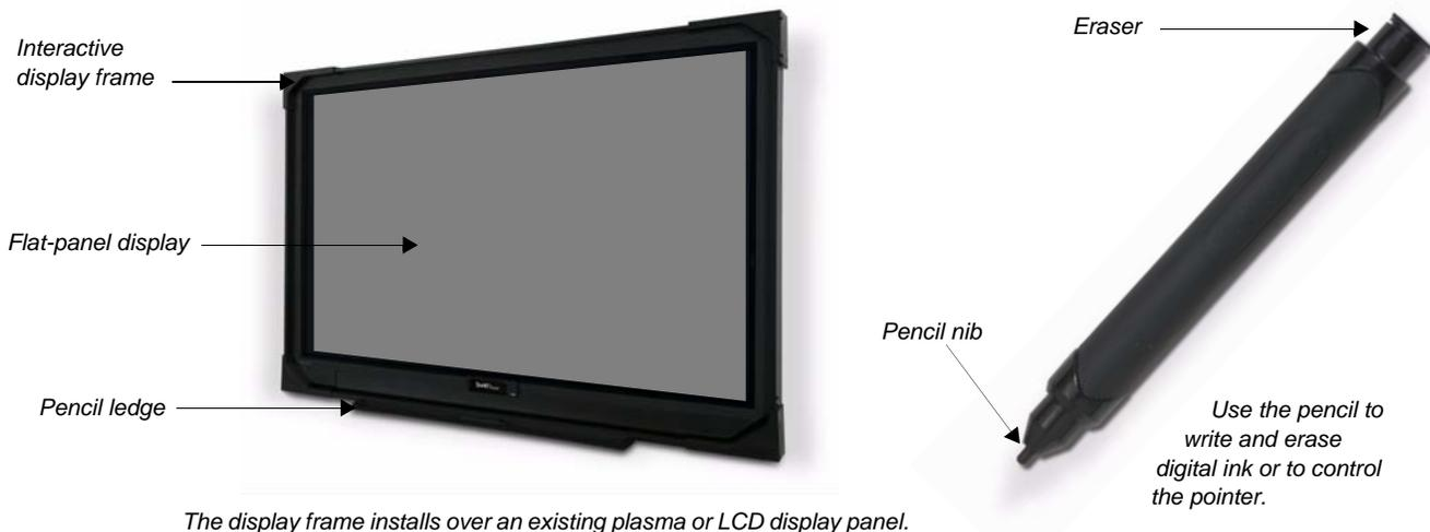
It may help you to think of your interactive display frame the same way you think of your mouse or keyboard – it is an input device that allows you to control applications on your computer. Digital cameras, located in the bottom corners of the interactive display frame, recognize the position of your finger or pencil on the surface of the display. You can control applications by touching the surface of the interactive display and you can use the pencil to write and erase digital ink.
