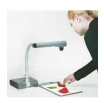
The SMART Document Camera uses a high-resolution video camera to display clear and detailed images in real time.
