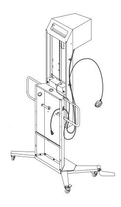
7. Bundle all cables between the HAWM-UX/UF and the FS-UX using zip ties, convoluted tubing, spiral wrap or expandable loom (not included). This is for operating safety and to prevent cables from getting caught in the height adjustment mechanism. Carefully test the movement of the unit, using the HAWM-UX/UF's mobility switch. Make sure the cables aren't taut at any range of the HAWM-UX/UF's movement. If they're still taut, repeat this procedure until you find a suitable length for the cables.
