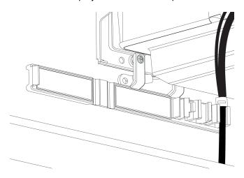
3. If the ECP is mounted on the left, place the WMB around the back of the HAWM-UX/UF, toward the left side of the interactive whiteboard. If the ECP is mounted on the right, place the WMB around the back of the HAWM-UX/UF toward the right side of the interactive whiteboard.
