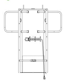
If you need to connect a peripheral device, guest computer or laptop to the interactive whiteboard system, make sure the cable is long enough so the computer or peripheral isn't pulled by the HAWM-UX/UF at its lowest or highest height. Attaching the laptop to the laptop shelf will ensure that this doesn't occur.
