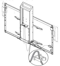
5. Bundle the excess cable, making sure that there is a minimum of 28" (71.1 cm) excess straight length or a 14" (35.6 cm) loose loop of cable.
