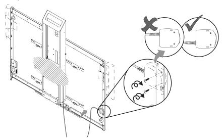
4. Place the cable through the HAWM-UX/UF's lower cable clip, making sure that the cable is taut between the interactive whiteboard and the clip, and loose between the clip and the base of the HAWM-UX/UF.
