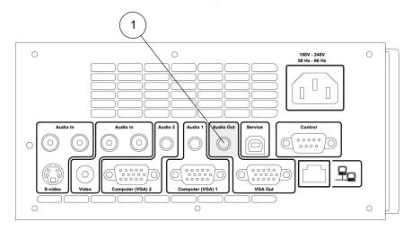
1. 3.5 mm audio-output connector (recommended for SBA/SBA-L speakers)
