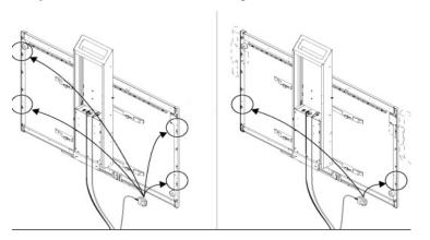
3. Secure the mobility switch cable toward the side of the interactive whiteboard where you chose to mount the mobility switch, using a Phillips No. 2 screwdriver and the two screws listed in the HAWM-UX/UF installation guide. Make sure that the cable is toward the bottom of the switch as you mount it.
