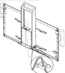
5. Bundle the excess cable, making sure that there's a minimum of 28" (71.1 cm) excess straight length or a 14" (35.6 cm) loose loop of cable.
