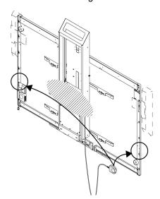
3. Secure the mobility switch cable using a Phillips No. 2 screwdriver and the two screws listed in the HAWM-UX/UF installation guide. Secure the mobility switch cable toward the side of the interactive whiteboard where you chose to mount the mobility switch. Make sure that the mobility switch cable is toward the bottom of the switch as you mount it.
