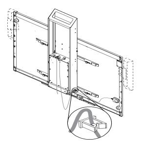
5. Bundle the excess cable, making sure that there's a minimum of 28" (71.1 cm) excess straight length or a 14" (35.6 cm) loose loop of cable.
