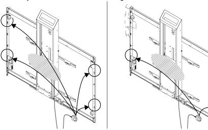
3. Secure the mobility switch cable using a Phillips® No. 2 screwdriver and the two screws listed inside the HAWM-UX/UF installation guide. Secure the mobility switch cable toward the side of the interactive whiteboard where you chose to mount the mobility switch, and make sure that the cable is toward the bottom of the switch as you mount it.
