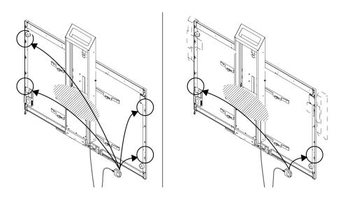
3. Secure the mobility switch cable using a Phillips No. 2 screwdriver and the two screws listed in the HAWM-UX/UF installation guide. Secure the mobility switch cable toward the side of the interactive whiteboard where you chose to mount the mobility switch and make sure that the mobility switch cable is toward the bottom of the switch as you mount it.
