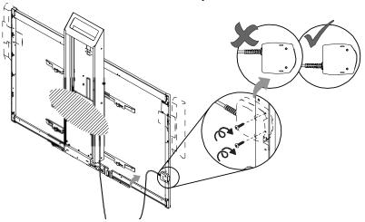
4. Place the cable through the HAWM-UX/UF's lower cable clip, making sure that the cable is taut between the interactive whiteboard and the clip, and loose between the clip and the base of the HAWM-UX/UF.
