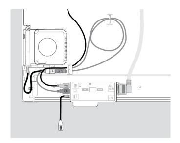
6. Use the WMB's magnetic connection to attach the WMB to a metal surface, until you need to attach a guest computer to it.
