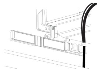
4. Place the WMB through the top cable clip you installed on the side of the HAWM-UX/UF.
