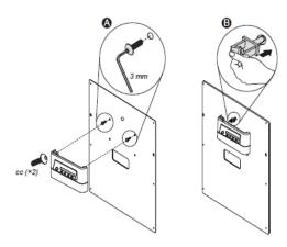
Flip up the bottom panel of the ECP. Attach two screws in the two bottom plastic anchors using a Phillips No. 2 screwdriver
