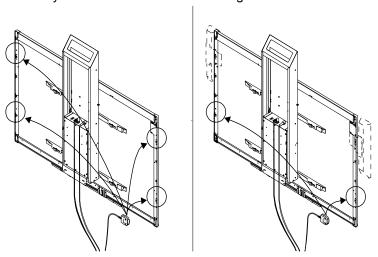
3. Secure the mobility switch cable using a Phillips® No. 2 screwdriver and the two screws listed inside the HAWM-UX/UF installation guide. Secure the cable toward the side of the interactive whiteboard where you chose to mount the mobility switch and make sure that the cable is toward the bottom of the switch as you mount it.
