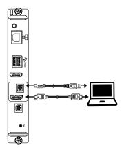
After you've connected the room computer to the AM30 appliance, you can use the Input app to switch to the room computer's desktop (see *Using Input* on page 27).
