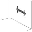
If the wall can't support the display's weight, you can use the SMART wall stand model WS-SBID-500 along with the SMART wall mount to transfer some of the weight from the wall to the floor. For more information about the SMART wall stand, see the *SMART wall stand installation instructions* (smarttech.com/kb/170466).
