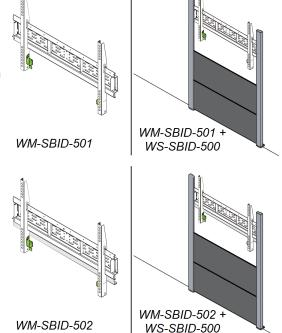
If you choose a third-party option rather than one of SMART's mounting options, be sure the wall mount can support the display's weight as well as the weight of any attached accessories and can accommodate the display's dimensions.
