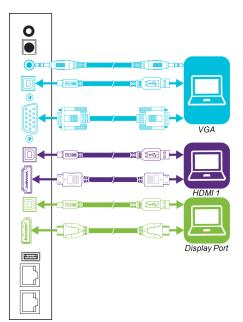
In addition to the three sets of computer connectors on the connector panel, there is one set of computer connectors on the convenience panel:
