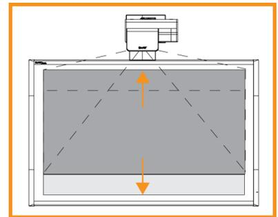
8. Adjust the scaling of the image by turning the yellow knob clockwise or counterclockwise to make the image larger or smaller on the interactive whiteboard.
