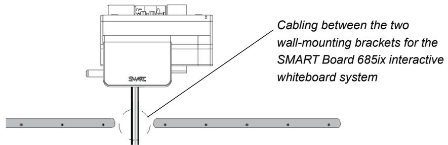
4. Space your peripheral cables equally and give the cables some slack between the wire management clip and projector. Close the latch on the wire management clip, ensuring that the cables aren't crossed.
