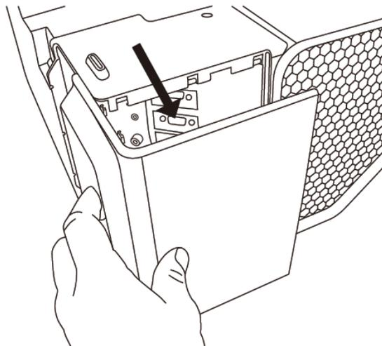
5. Release the latch on the wire management clip attached to the projector's wall-mounting bracket, beneath the projector.
