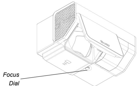
**Aligning the Image After Installation**
