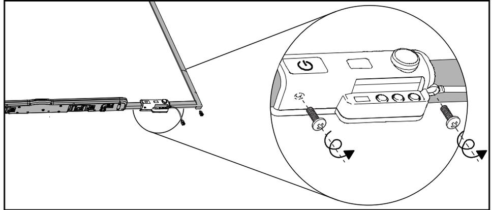
4. Locate the jumper cover on the side of the ECP that faces the wall, between the “PC” and “SE240” labels.
