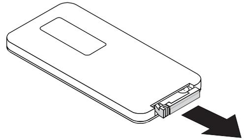
3. Insert a CR2025 coin cell battery into the battery holder.
