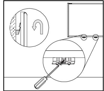
3. Align the pen tray with the two L-shaped metal brackets, and then slide it toward the wall until it rests snugly against the bottom frame of your interactive whiteboard.
