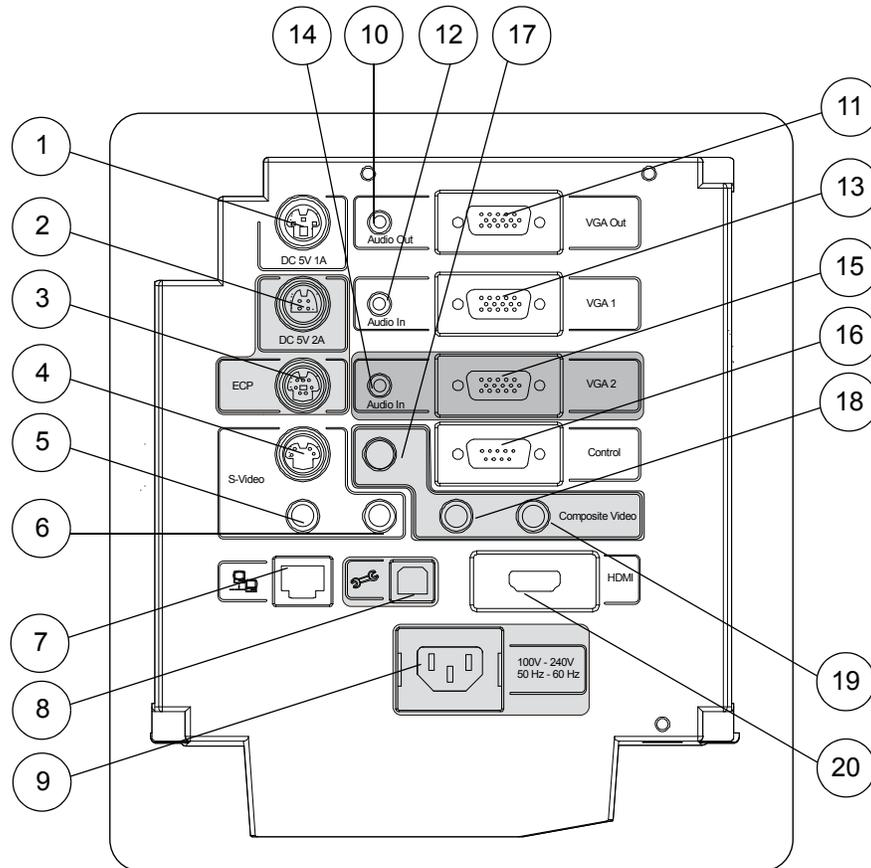
1. 3-pin mini-DIN 5V/1A connector
