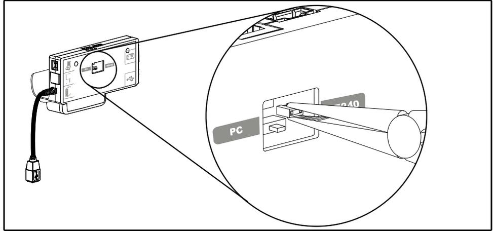
4. Insert the USB jumper cover into the USB A port on the front of the ECP.
