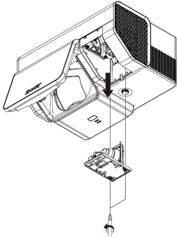
**To put the new lamp module into the projector**
