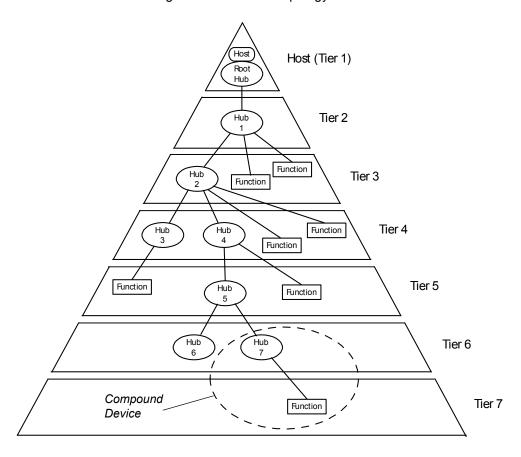
Timing constraints for hub and cable propagation times allow a maximum of seven tiers, including the root tier. In seven tiers, a maximum of five non-root hubs can be supported in a communication path between the host and any device. Note that a compound device occupies two tiers; therefore, it cannot be attached at tier seven where only functions can be used.
