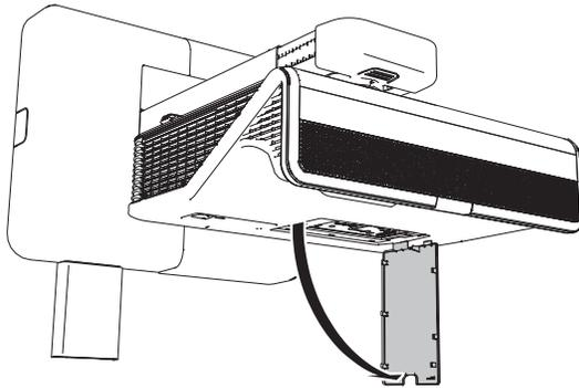
5. Use a Phillips screwdriver to loosen the two captive screws from the bottom of the lamp module.
