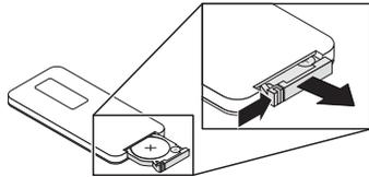
2. Remove the old battery from the battery holder and replace it with a CR2025 coin-cell battery.
