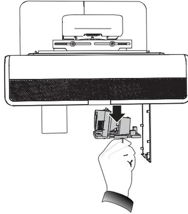
**To put the new lamp module into the projector**
