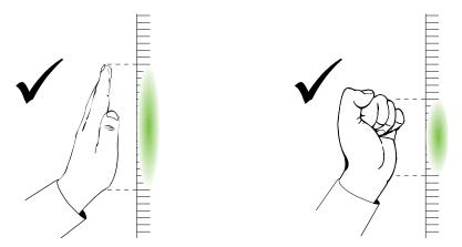
When using the pen tray's eraser, use the wide surface for large areas, and the smaller, angled surface for smaller areas. Don't use the edge of the eraser because this could be interpreted incorrectly.
