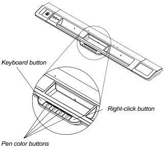
Pressing the Keyboard and Right-click buttons simultaneously starts the orientation process.
