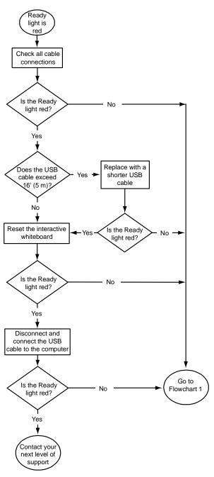
The interactive whiteboard is connected to your computer with a USB cable and to the wall outlet with a power cable. You can access these cables by reaching under the pen tray.
