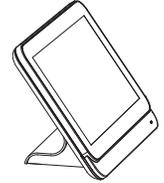
The console is typically located on the meeting room table. Like the interactive flat panels, the console features a 16:9 LCD screen with touch technology, and you can interact with buttons and other controls by pressing them.
