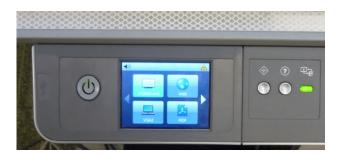
**Note:** The interactive display does not have an ACP. Instead, you control the appliance settings on-screen through the software interface.
