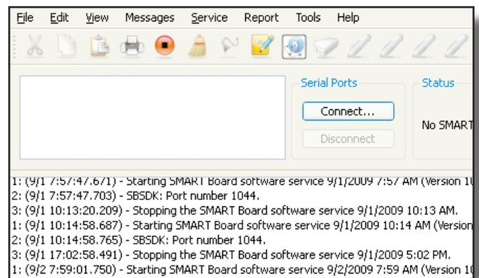
You can find important diagnostic information in the log window. The log registers all of the information that is sent to and from the interactive product. This includes hardware information such as the detection of the pen tray, and software information – such as the firmware version number. SMART Technical Support will often ask you for this information when diagnosing and troubleshooting your interactive product issues.
